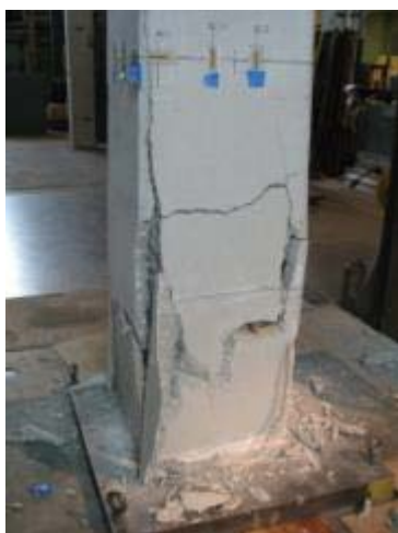
Fig. 5: Specimen B-3: normalized axial stress-normalized axial deformation response where the thick line shows the envelope curve (a); photograph of failed specimen (b); close-up of failed GFRP tie and bulged bar (c).
