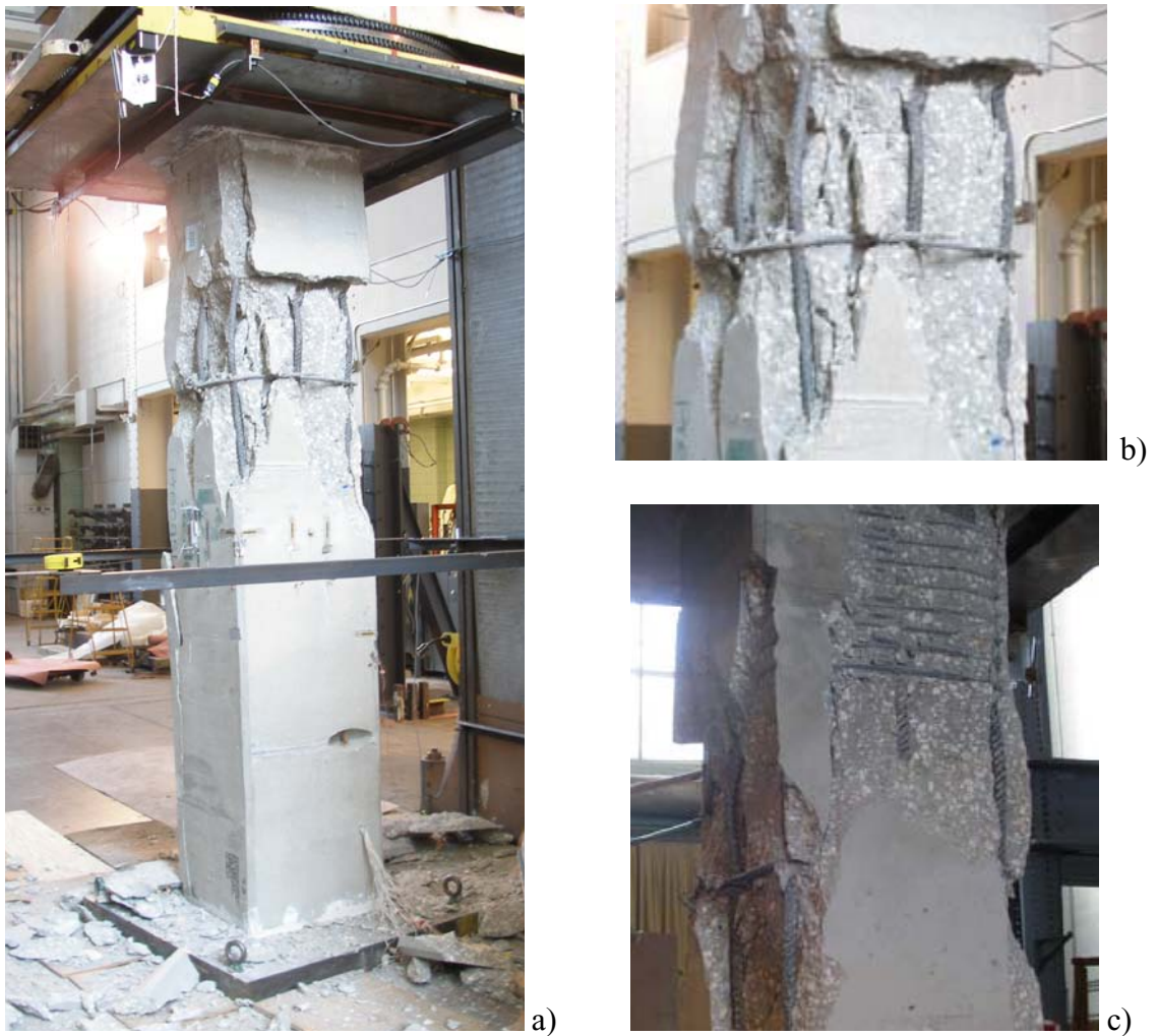
Fig. A - 22: Failure of Specimen S-1-control (a-c).
