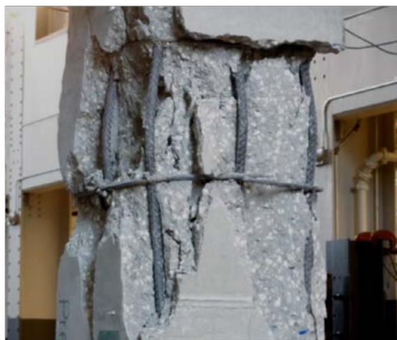
Fig. 3: Specimen S-16: normalized axial stress-normalized axial deformation response where the thick line shows the envelope curve (a); photograph of failed specimen (b); close-up of buckled steel bars (c).
