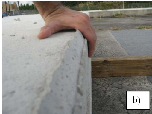
Fig. A - 4: Chamfering of the corners: grinding of the corner (a); corner before chamfering (b); corner after chamfering (c).
