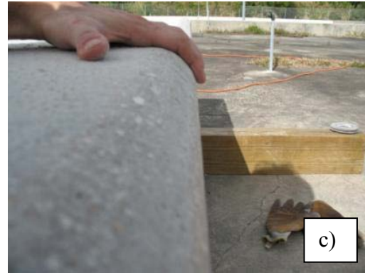
Fig. A - 4: Chamfering of the corners: grinding of the corner (a); corner before chamfering (b); corner after chamfering (c).
