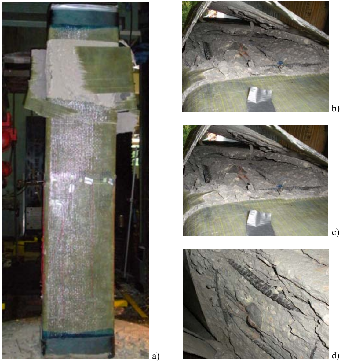
Fig. A - 24: Failure of Specimen S-1-2GB (a-d).
