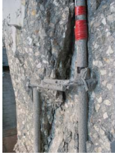
Fig. A - 19: Failure of Specimen B-12 (a-d).
