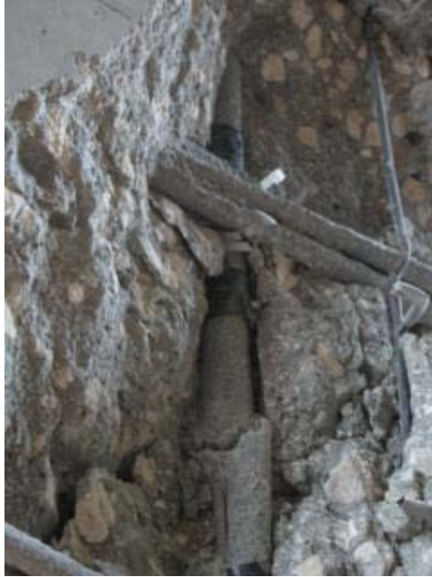
Fig. A - 19: Failure of Specimen B-12 (a-d).
