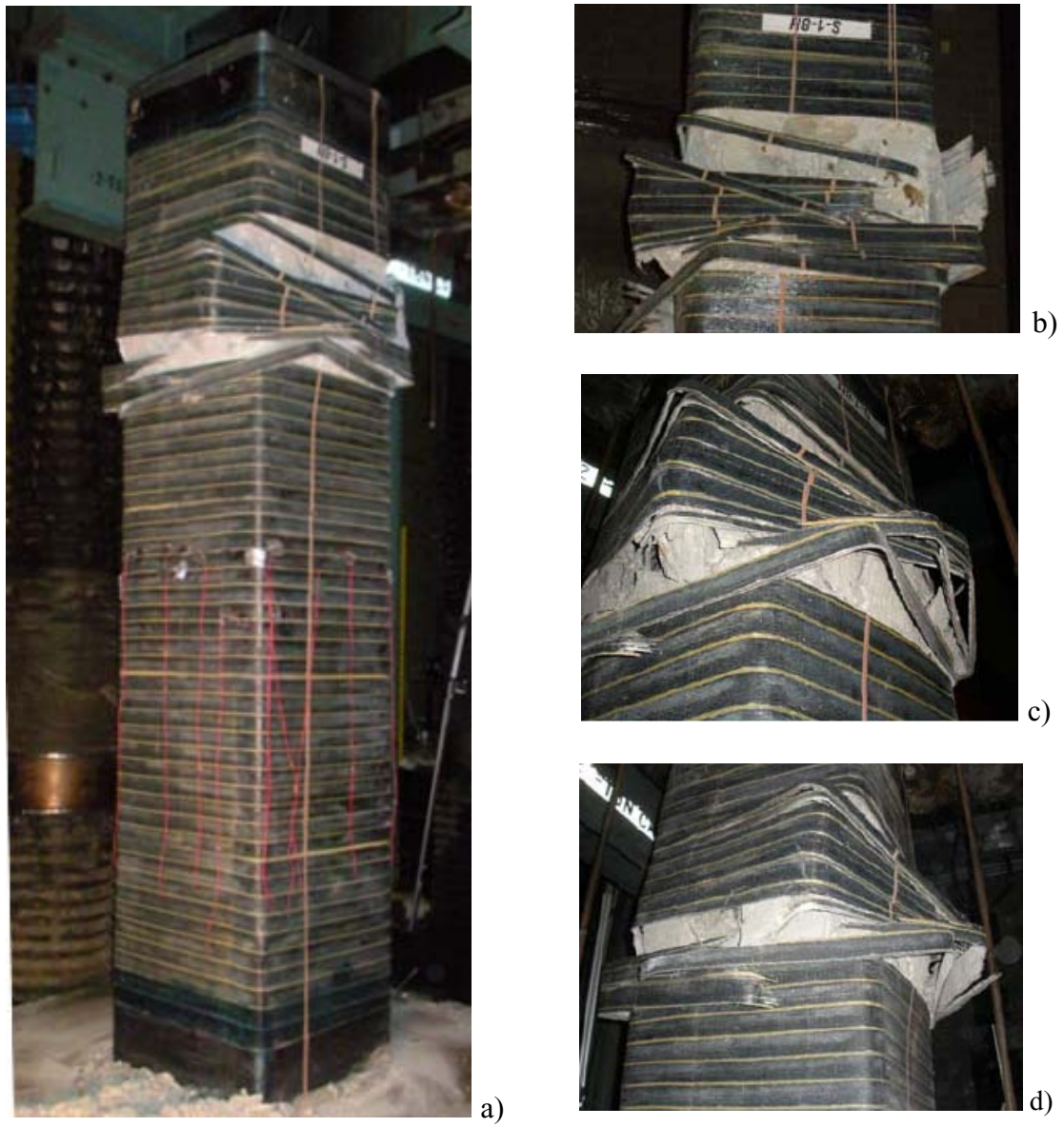
Fig. A - 25: Failure of Specimen S-1-8H (a-d).
